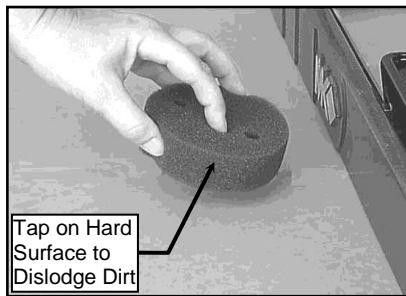
(E) Clean Filter by Tapping on Hard Surface or using Compressed Air
